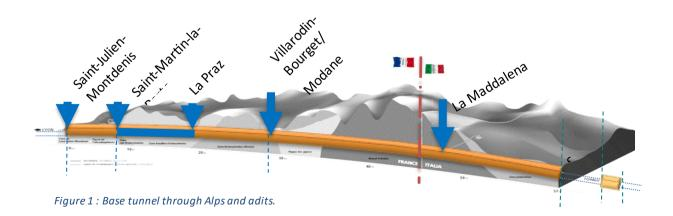
The Mont-Cenis base tunnel is a complete geological section of the Western Alps, which are crossed from west to east with an overburden of over 2,000 metres.
