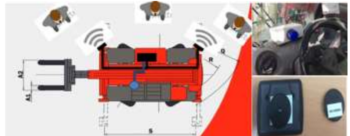
Figure 7: Application of RFID, with details of cab alarm (top right) and the tag/badge wearable by workers (bottom right).
