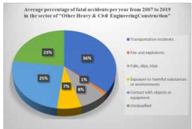
Figure 1: accident statistics from DOL OSHA in "Other Heavy and Civil Engineering Construction" (which includes tunnel construction) classified by event or exposure.
