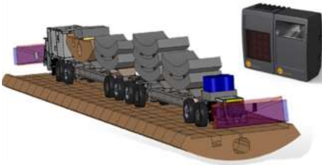
Figure 8: wheeled trucks for prefabricated segments transport, equipped with infrared sensor system.
