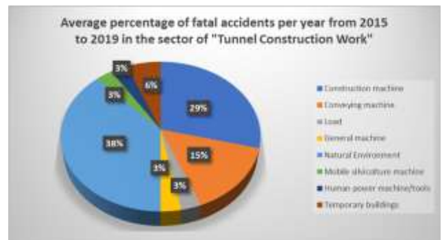
Figure 2: accident statistics from JISHA in "Tunnel Construction Work" classified by event or exposure.
