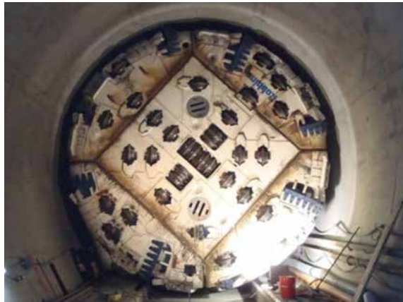
Figure 2 - Gea, the Maddalena exploratory tunnel TBM
