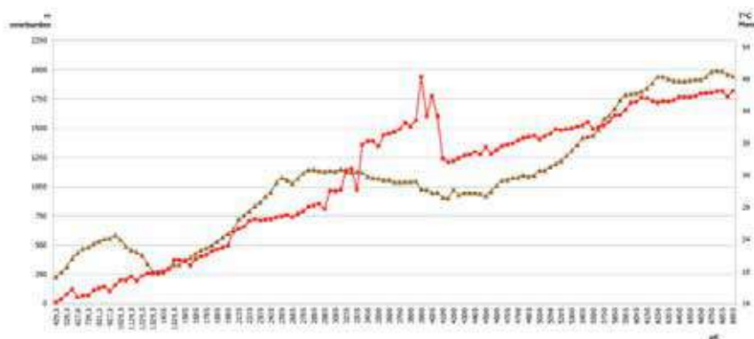
Figure 10 – Rock mass temperature according to overburden along the tunnel (data from mobile stations)
