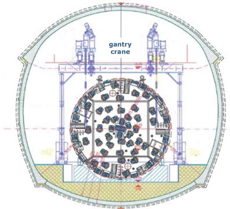
Fig. 3. The assembly cavern with a view of the gantry crane and the TBM head.
