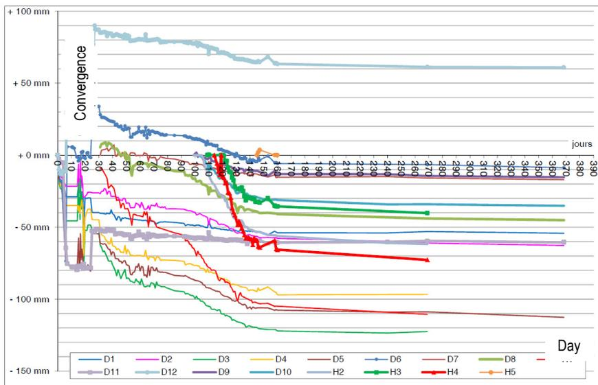
Fig. 10. Convergence monitoring system (a). Typical convergence history along selected lines, D1 to D9 and H1 to H5 (b)
