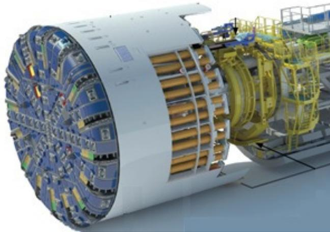
Fig. 2. TBM « Federica » used for excavation of the South Base Tunnel (9 km long) between Saint Martin La Porte and La Praz.
