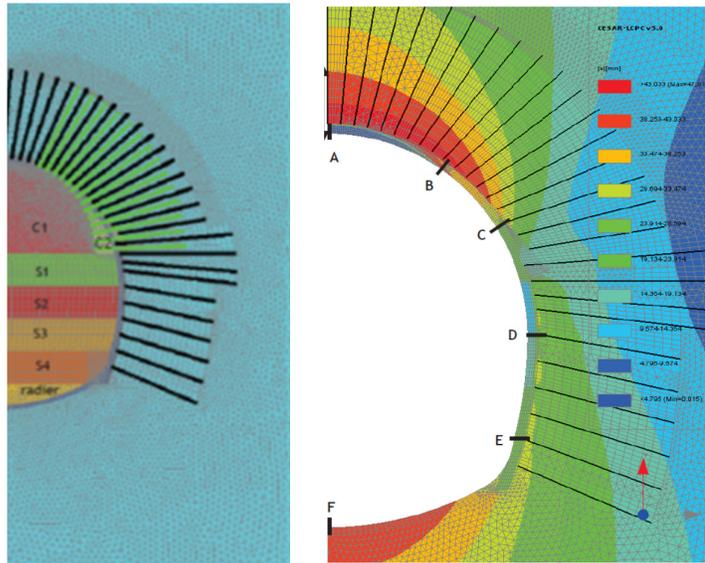
Fig. 6. FEM model showing the excavation support stages simulated (on the left). Displacement distribution at the end of the excavation and reinforcement simulation process (on the right).
