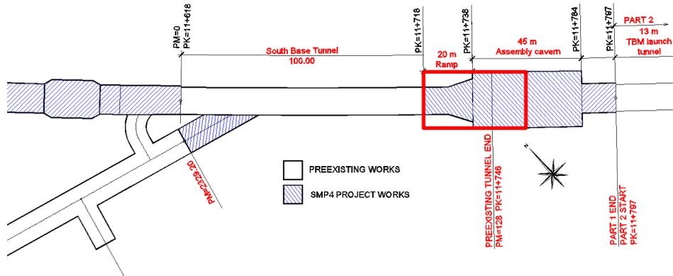
Fig. 4. Plan view of the Assembly Cavern. The red box shows the locations finally chosen.
