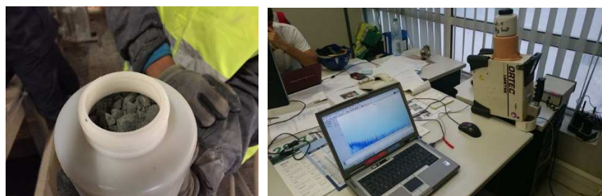
Figure 10. Measuring equipment in the on-site laboratory measuring the radioactivity of the sample (0/40 SMP4)
